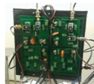
Test board used at Texas A&M University Cyclotron Facility
