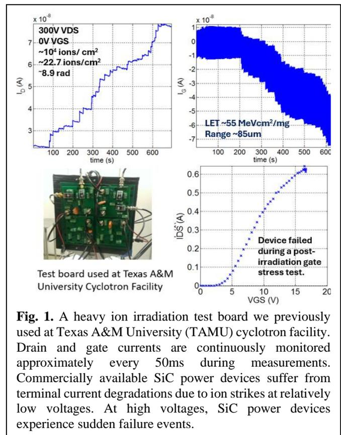
**Fig. 1.** A heavy ion irradiation test board we previously used at Texas A&M University (TAMU) cyclotron facility. Drain and gate currents are continuously monitored approximately every 50ms during measurements. Commercially available SiC power devices suffer from terminal current degradations due to ion strikes at relatively low voltages. At high voltages, SiC power devices experience sudden failure events.
