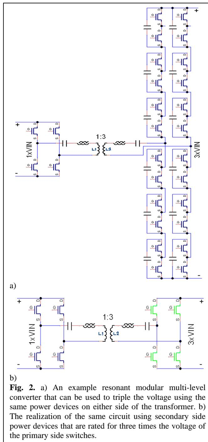
**Fig. 2.** a) An example resonant modular multi-level converter that can be used to triple the voltage using the same power devices on either side of the transformer. b) The realization of the same circuit using secondary side power devices that are rated for three times the voltage of the primary side switches.
