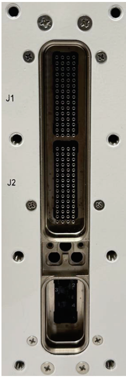
Figure 5: Exterior of the unit showing ARINC 600 receptacle
