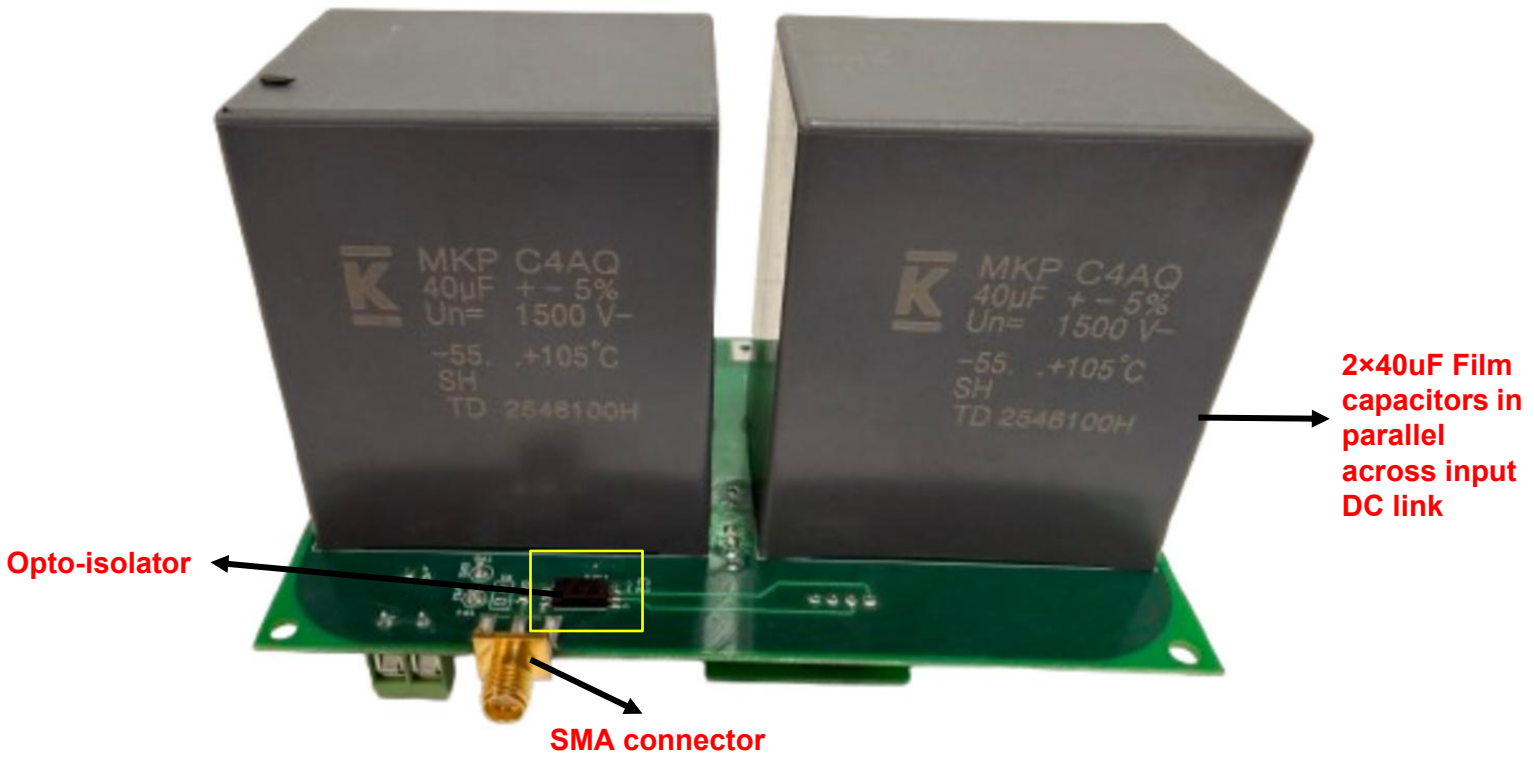
Figure 2 : SCT evaluation board: Down-side view with components.
