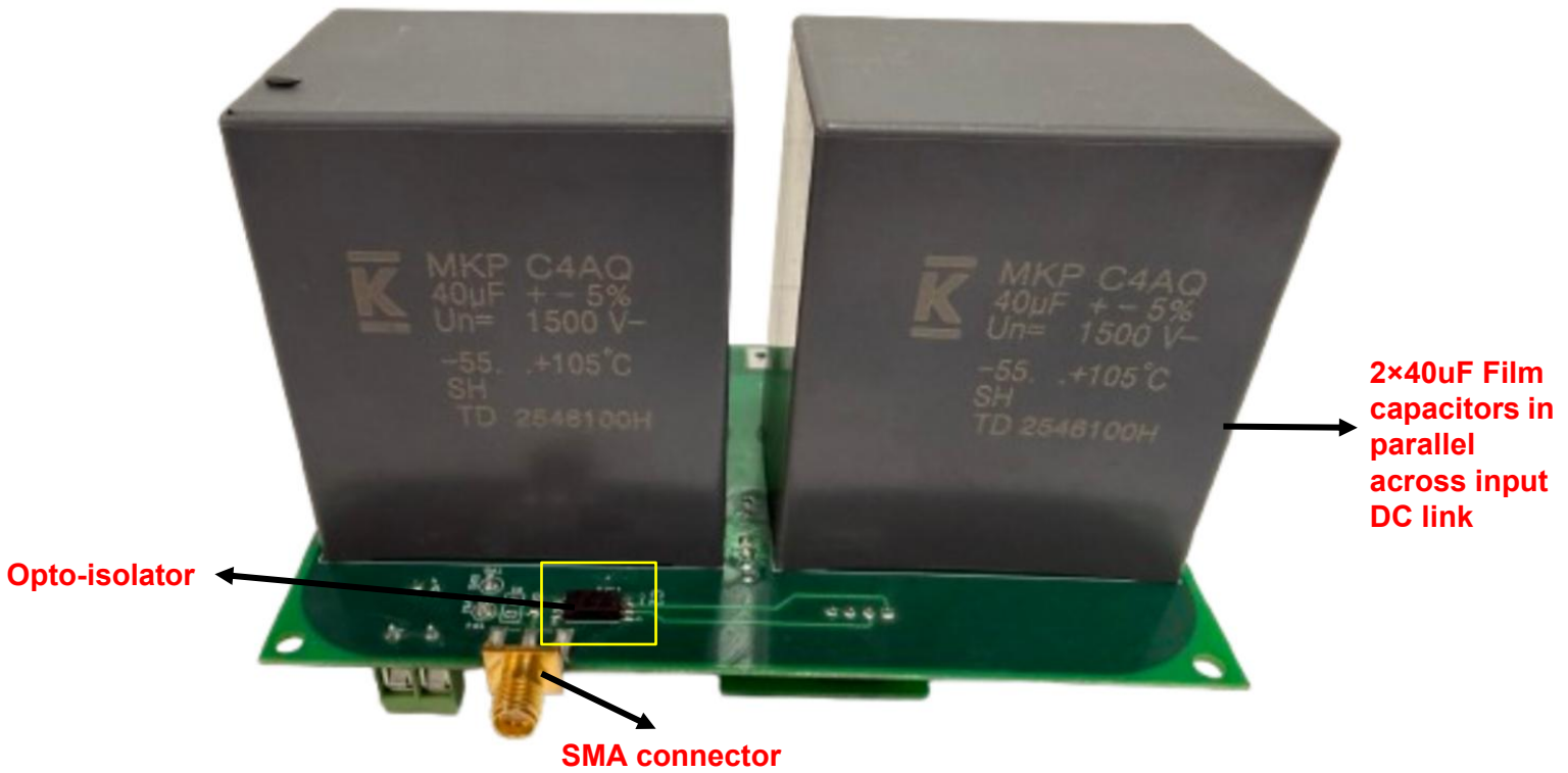
Figure 2 : SCT evaluation board: Down-side view with components.
