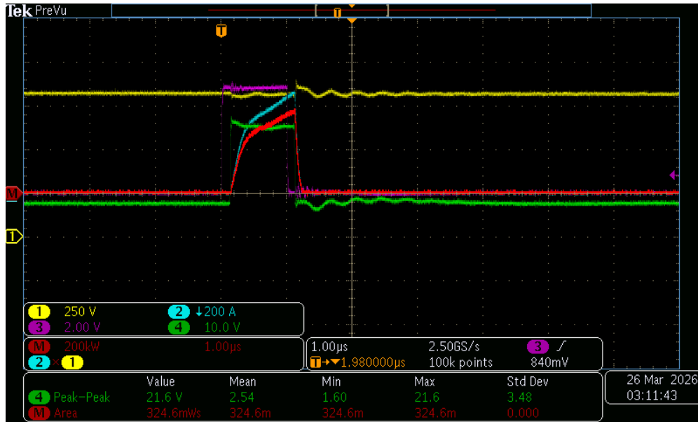
Figure 8: Oscilloscope waveform obtained during an 800V SCT with a 1 \mu s pulse
