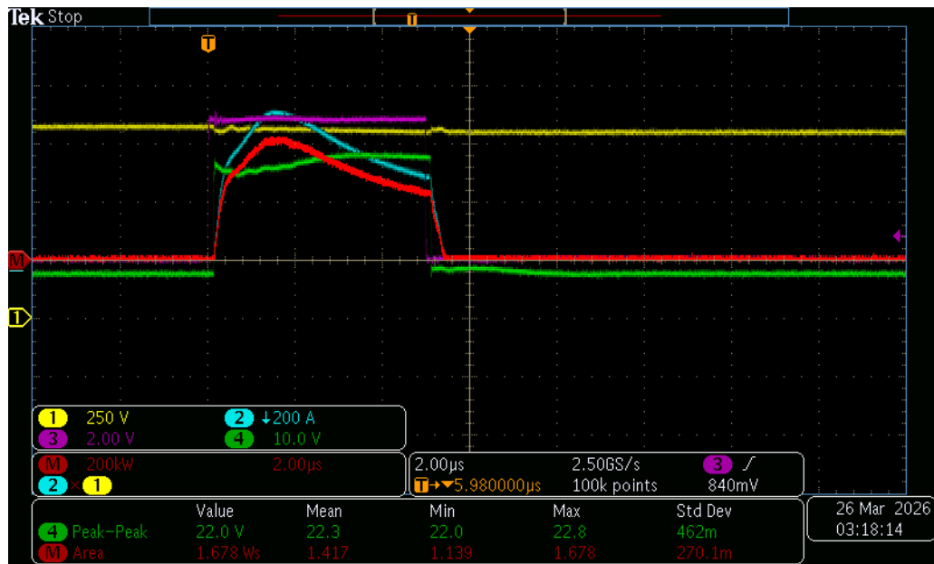
Figure 12: Oscilloscope waveform obtained during an 800V SCT with a 5µs pulse
