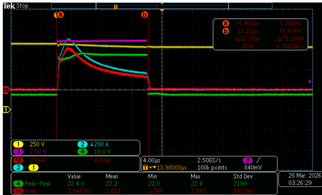
Figure 18: Oscilloscope waveform obtained during an 800V SCT with a 12µs pulse
