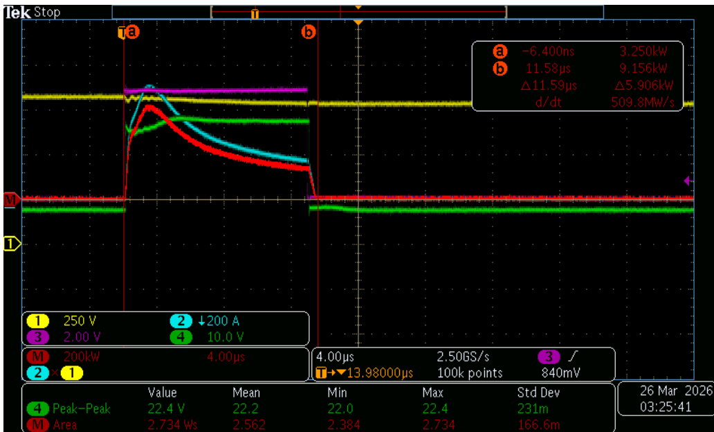
Figure 17: Oscilloscope waveform obtained during an 800V SCT with a 11µs pulse
