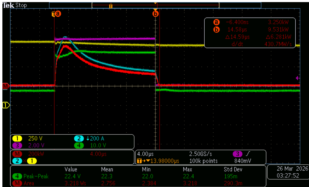
Figure 20: Oscilloscope waveform obtained during an 800V SCT with a 14µs pulse
