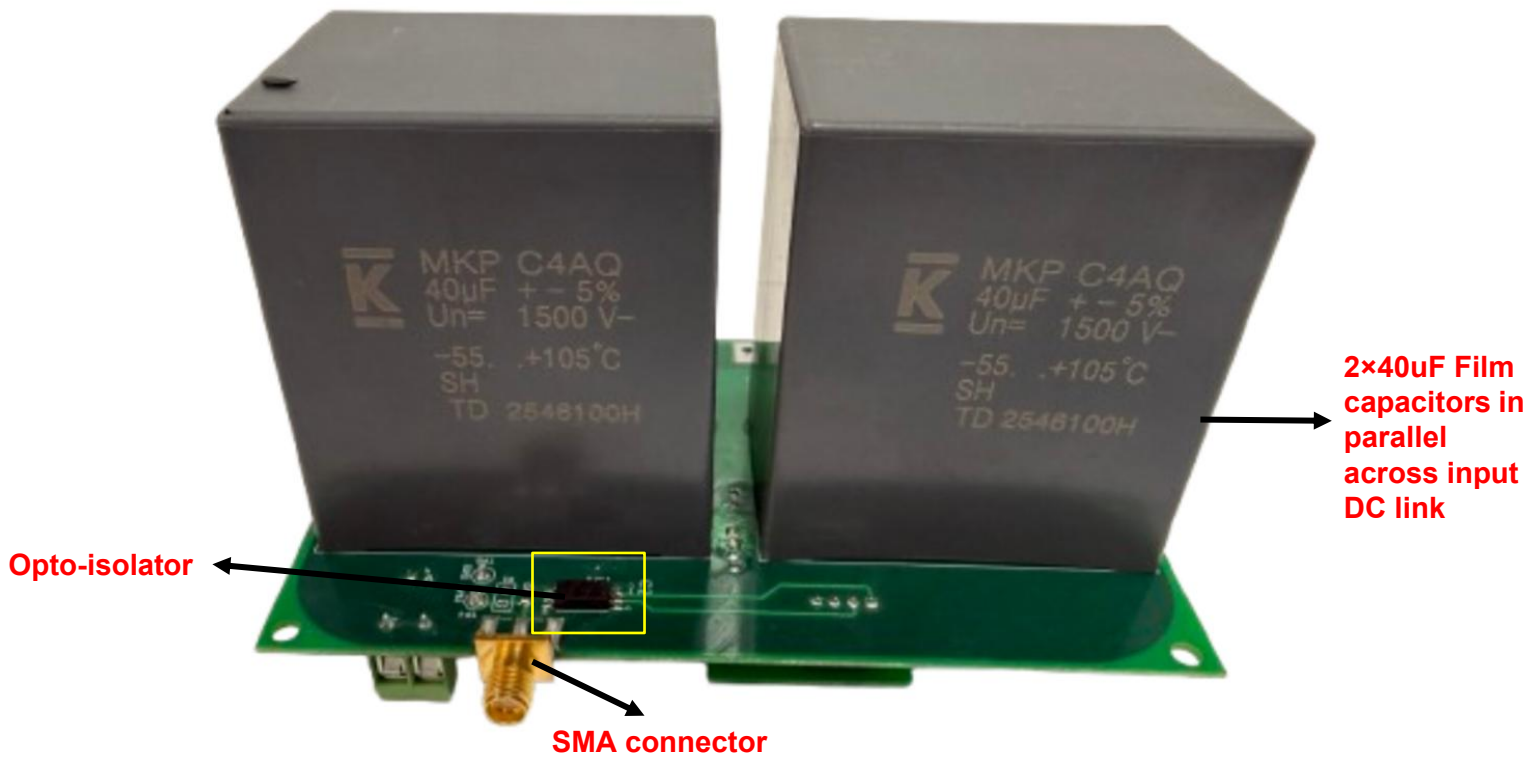
Figure 2 : SCT evaluation board: Down-side view with components.
